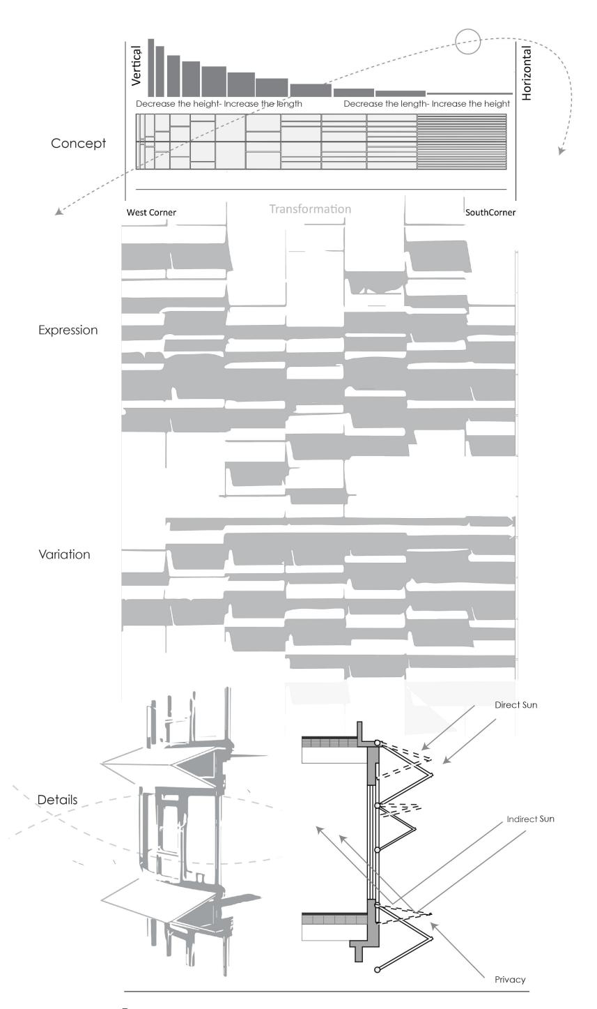
The Aluminum framed double layer curtain wall is a automated transformable screen. The concept of the screen is developed based on the solar radiation. The southeast side of the screen has horizontal louvers and it transformed its width to length in a way that it gets more vertical in size towards south west corner. The screen will be controlled by the user of the room, and the variation movement of the screen will also create a impression of living b u i l d i n g
