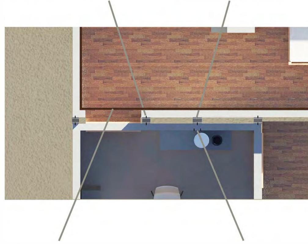
This is a wood veneer molding at a right angle between the wall and ceiling. This will help eliminate any leakage into the caravan and also give the interior a more traditional aesthetic. The same wood veneer may be used to frame windows in the caravan to minimize leakage and provide a similar traditional aesthetic. Open shelving is hung on the structural wall in order to ensure stability. The shelves are screwed in where the beam meets the wall.
