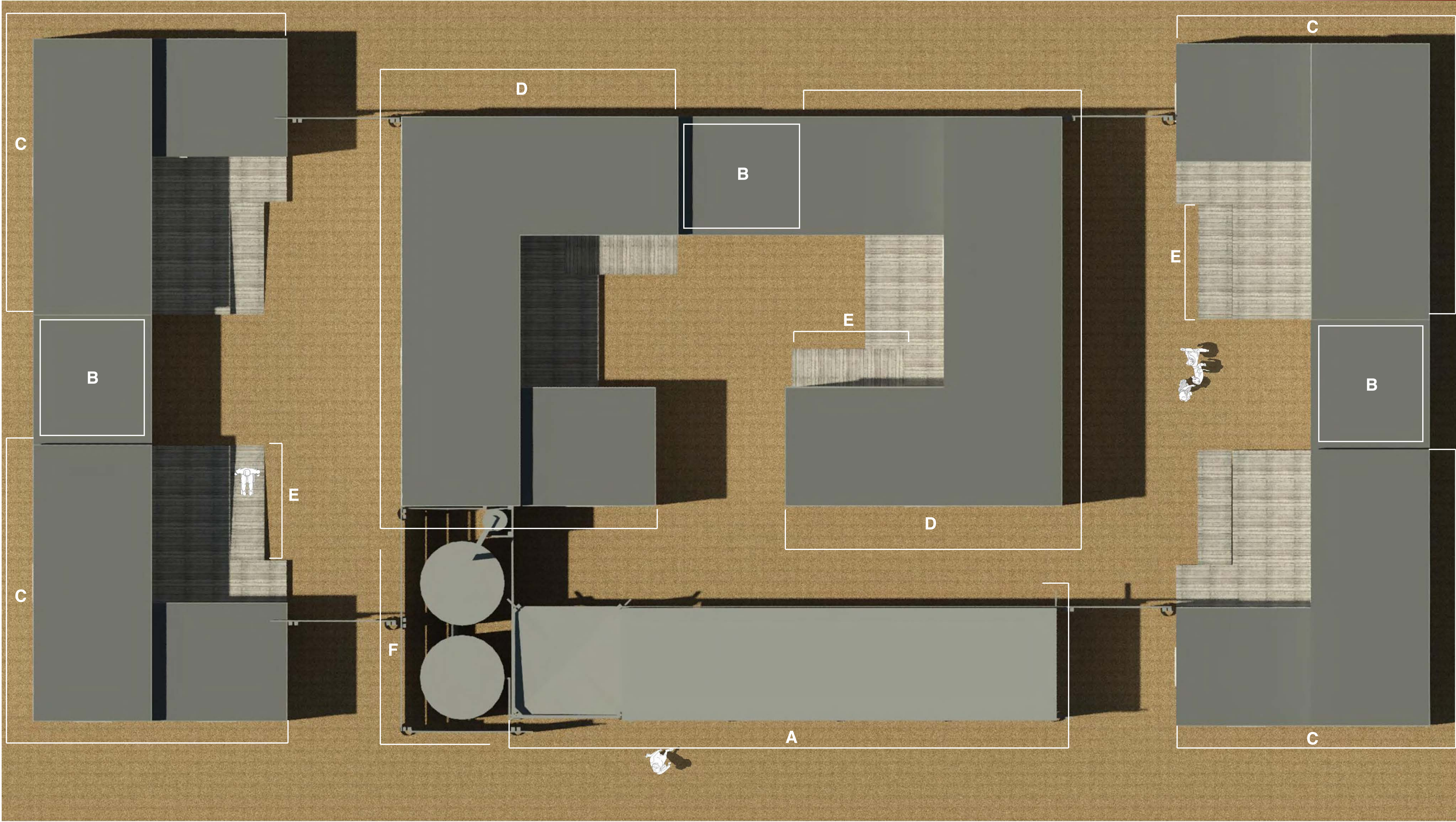
A) Communal Structure B) Split Caravans transformed into bathrooms C) "L" Shaped Caravan Home D) "U" Shaped Caravan Home E) Ramp F) Enclosed Rainwater Tanks
