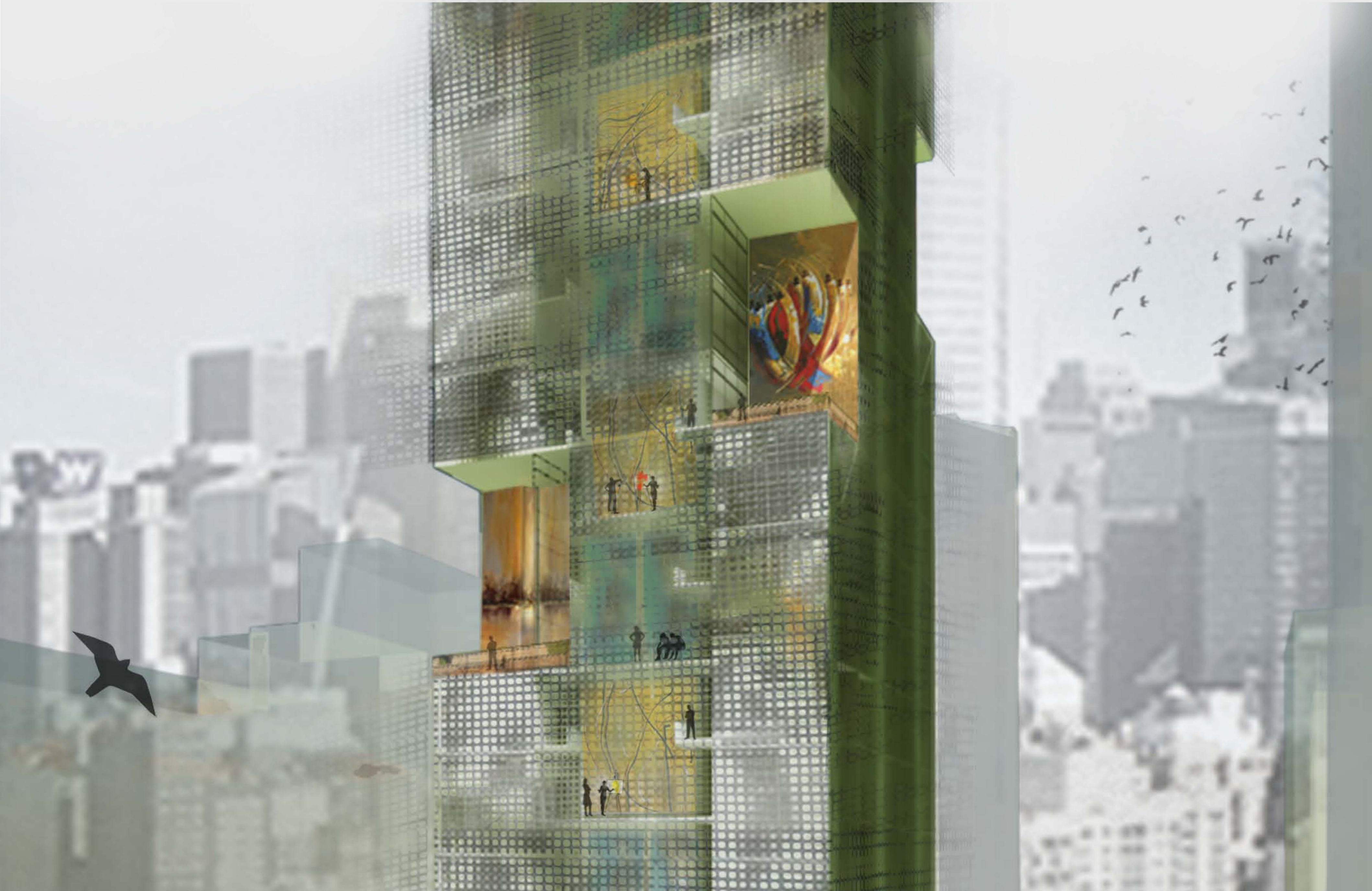
school of visual arts : 3d view showing the almost transparent fritted glass screen and the urban apertures crawling up the tower; the double height common workspaces and interaction spaces
