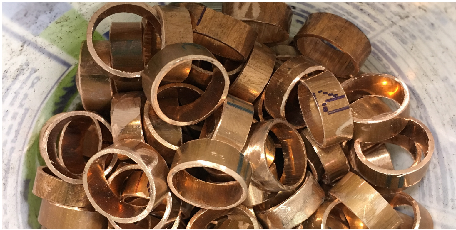
Cut-off copper pipe end pieces were cut into 1/4" spacers for the steel frames.
