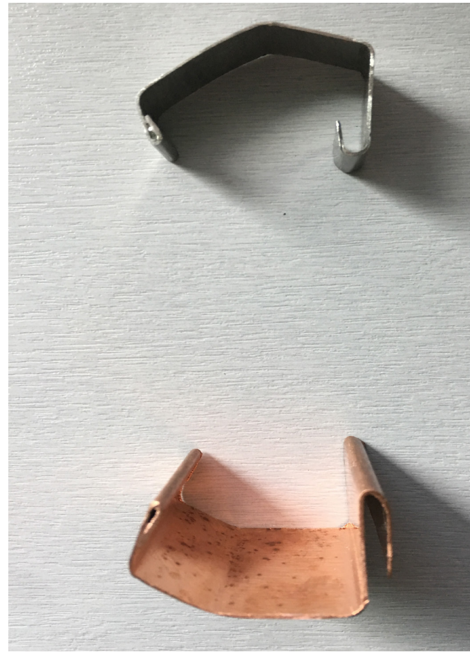
Custom copper and stainless steel profiles were created and cut into more than 2,000 clips to fasten the tile to the armature.
