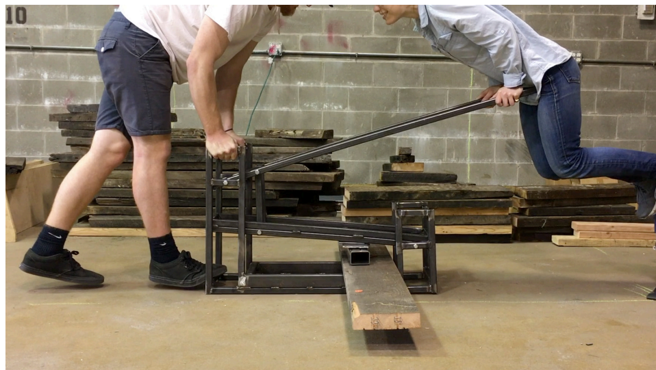
Apply weight to the lever arm of the press until you hear a crunching sound.
